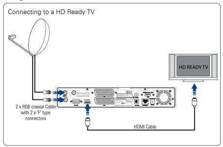
Connect two RG6 co-axial cables fitted with 'F' type connectors from your satellite dish to the 'TUNER1' and 'TUNER2' sockets on the back panel of your Digital TV Recorder.
